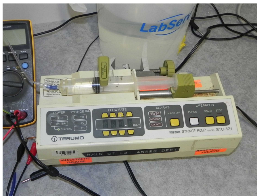
Figure A.7: Photo of the syringe pump used to produce drops and control flow rate.
