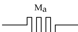
Figure 7.9: Electrical symbol of a memristor, as is used in the original electrode-electrolyte interface model
