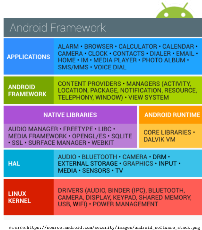
Figure 2.7: Android software stack [26].
