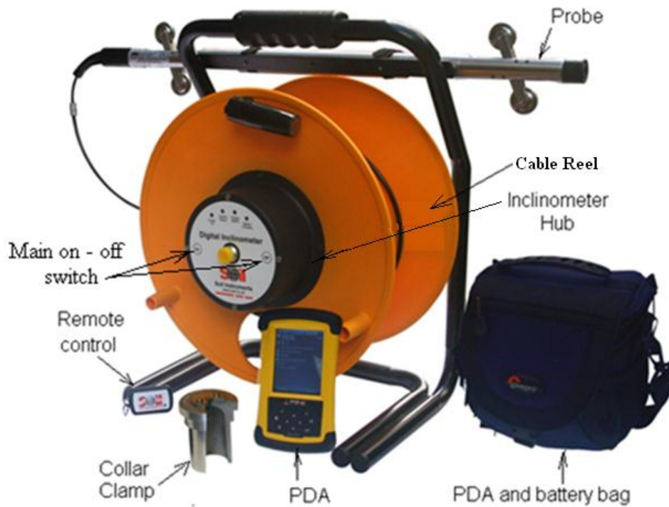
Figure 4.6 Digital Inclined Inclinometer system (from SOIL, 2008).
