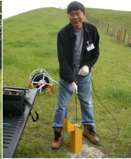
Figure 4.5 Inclinometer monitoring photo two (Photo: Page, 2011).
