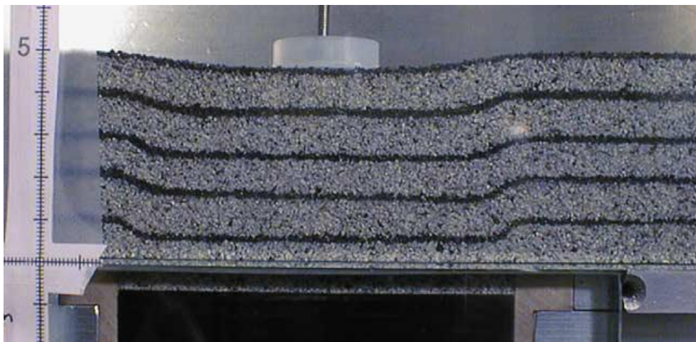
Figure A 23 Axisymmetric trap-door mechanism in small-scale model test with dry sand (Vardoulakis et al. 2004).
