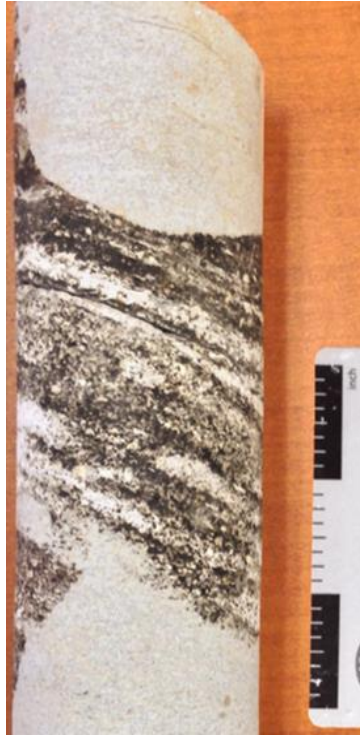
Figure 5.7. Fabric concordant and discordant oil-saturation geometries in core of Haney Limestone <50-ft depth taken from Stampede Asphalt Rock Mine in Logan County, Kentucky. Fabric discordant calcite is the latest calcite generation. For location see Figure 2.4.
