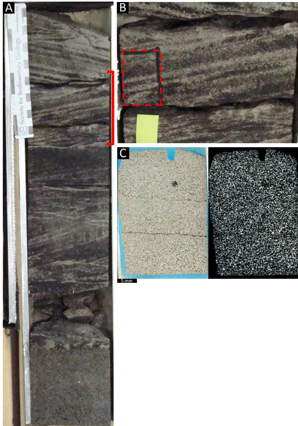
Figure B.16. MegaWest Core 109 core 1 box 4. A) Box of core. B) Sampled location in core. C) Scanned thin section under plane-polarized (left) and cross-polarized light (right). Thin section of sample 109c1-b4 is of standard, 30 \mu\text{m} thickness.
