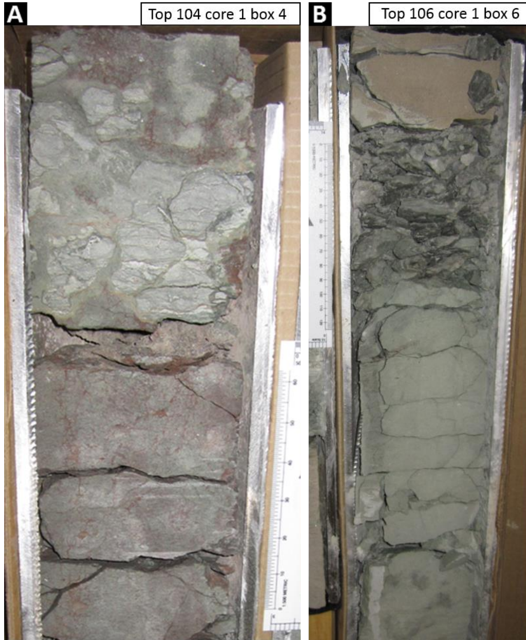
Figure 5.2. Evidence of exposure prior to burial in unsampled core section from cores 104 and 106. Scale bar in both images is in centimeters. A) Pebble- to cobble-sized blocks of calcareous mudstone suspended in a green glauconitic cement crosscut by siderite veinlets in Core 104 core 1 box 4. Exposure surface is approximately 16 \pm 3 ft above sampled section of 104c1-b10 (466-ft elevation). B) Glauconitic shale and siltstone with calcareous cobbles in Core 106 core 1 box 6.
