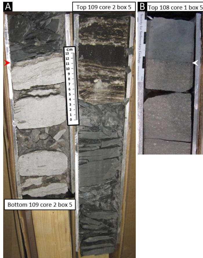
Figure A.15. Difference in sandstone contacts. A) Big Clifty and Beech Creek (Barlow) Limestone contact (red arrowhead) from Core 109, scale along box divider is in centimeters. Lithology transitions from sandstone to shale to wackestone down hole. B) Hardinsburg and Haney contact (white arrowhead) from Core 108, scale left of core is in inches. The Hardinsburg (above the white arrowhead) is a clean sandstone while the Haney (below the white arrowhead), is a crinoidal grainstone. The core was wetted with water prior to photographing.
