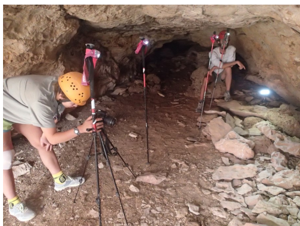
Figure 1: Image of an entrance area photogrammetry set up at GRCA. To reduce the amount of equipment brought into the cave, the authors use trekking poles and caving lights to illuminate the site.
