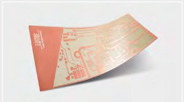
Semi-Flex material, Cu layer thickness 18  $\mu\text{m}$
