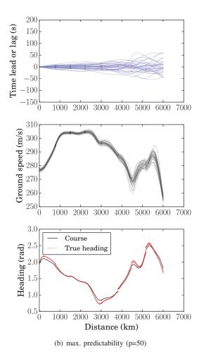
Figure 4. State-space evolution of the variables in the case p = 0 and p = 50. Time leads and lags are defined with respect to the average trajectory.
