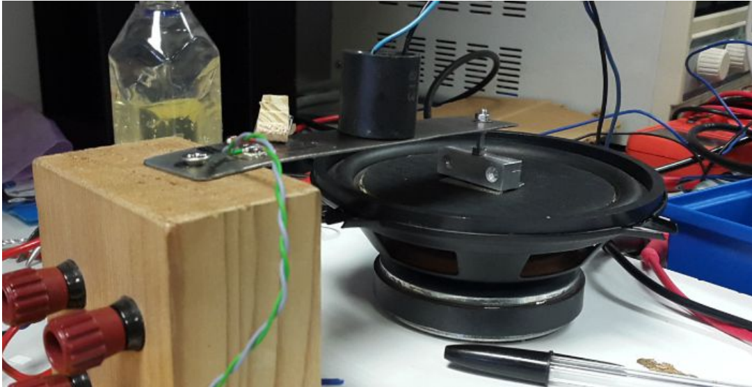
Figure 26: Ultrasonic transducer placed in metal plate with PVDF and strain gauge
