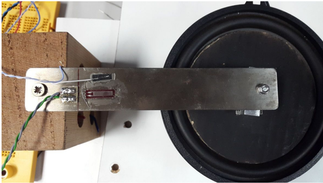
Figure 25: Steel metal plate with PVDF and strain gauge connected to speaker
