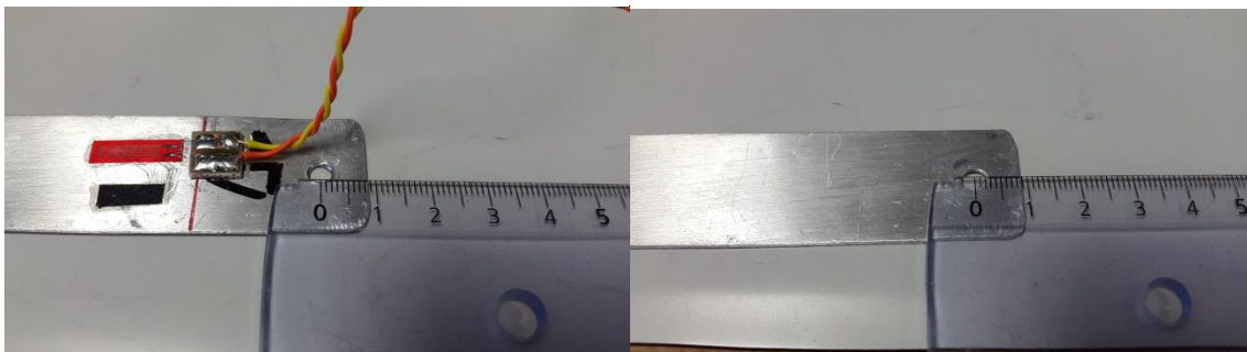
Figures 21 and 22: Dimensions of the holes drilled in the metal plates
