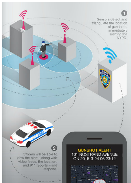
Figure 2.8: Real-time gunshot detection bounds the area where the shot was heard and notifies the 911.
