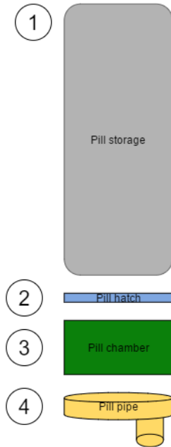
Figure 26: Pillbox refilling mechanism schematic
