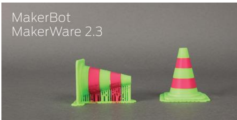
Figure 73: Example of printing a cone in a standing position and in a side position, the standing position does not need any extra support structures while the sideways position does
