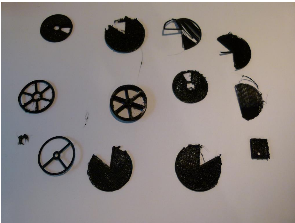
Figure 74: Discarded parts due to their lack of quality or just printed as test parts.
