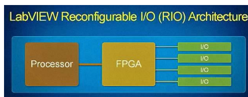
Figure 28. LabVIEW Reconfigurable I/O Arquitecure
