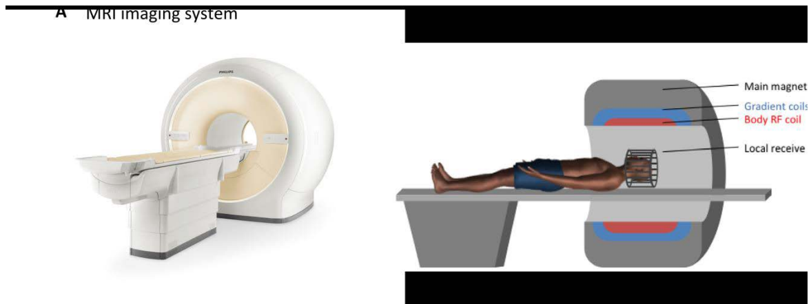
Figure 3: (a) State-of-the art MRI scanner (b) sketch of the main MRI hardware components taken from (18): main magnet, linear field gradient, RF system
