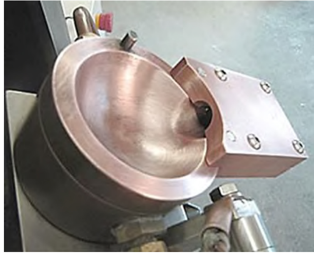
Figure 3.1: Copper casting module attached to the water-cooled copper crucible in the Arc 200 Mini Vacuum Arc Melter from Arcast Inc.
