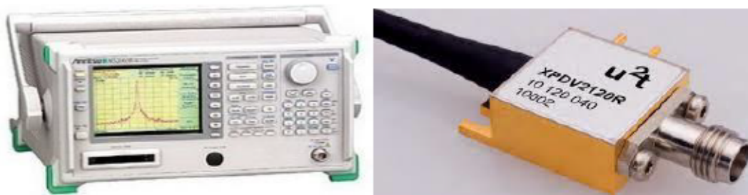
Figure 2.10. (a) Anritsu MS2668C Electrical spectrum analyzer. (b) U2T XPDV2120R PIN photodiode
