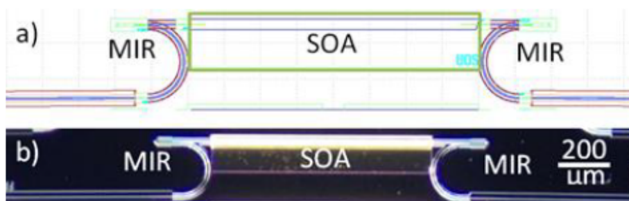
Figure 3.7. On-chip Fabry–Perot laser structures.(a) Structure of the oc-FP. (b) Microscope photograph of the oc-FP.
