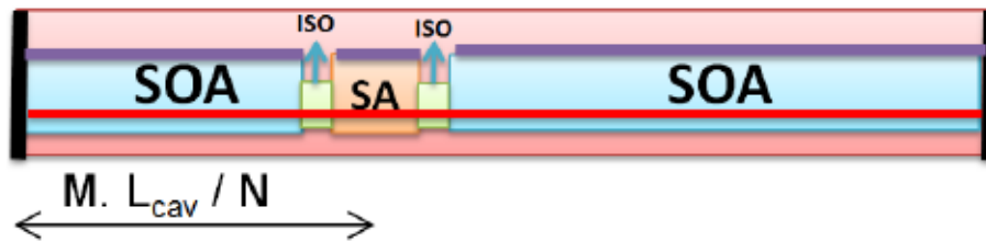
Figure 6.2. Asymmetric colliding pulse mode-locked structure, M \cdot L_{cav}/N , M and N are relative prime ( M < N )
