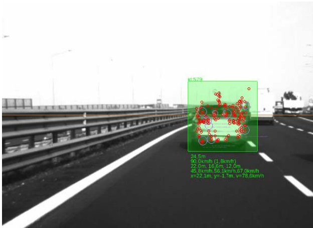
Fig. 2. Example of vehicle detection(green) and feature detection(red circles).
