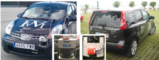
Figure 2. IVVI 2.0 platform with a detail of the laser scanner used and the inertial sensor used.
