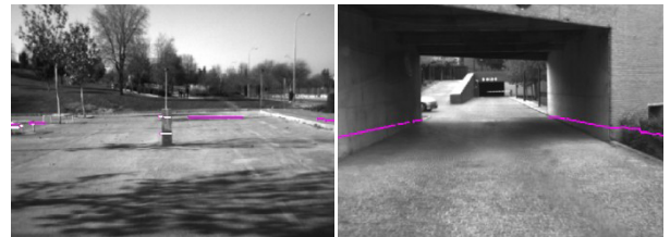
Figure 5. Laser scanner detections extrapolated to the camera with accurate precision.
