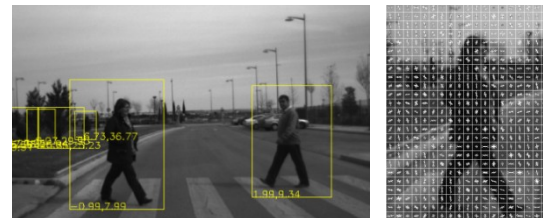
Figure 6. Examples of region of interest creation (left), with the distances to them highlighted, and HOG features calculation in a ROI (right).
