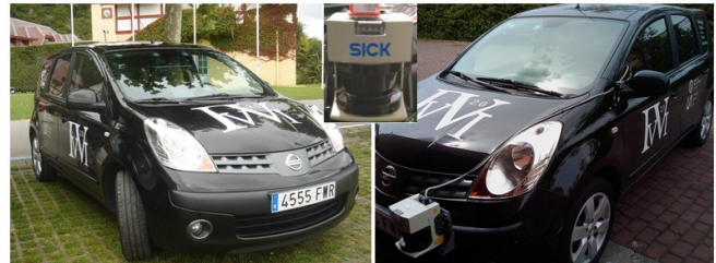
Figure 1. Test platform IVVI 2.0. (Intelligent Vehicle based on Visual Information). Left the vehicle. Right the laser scanner mounted in the bumper of the vehicle. Center, closer look of the laser scanner sensor.
