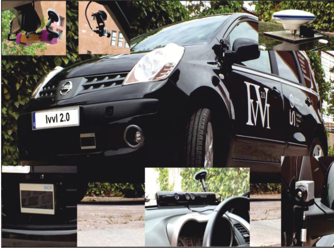
Fig. 1. Test vehicle IVVI 2.0.
