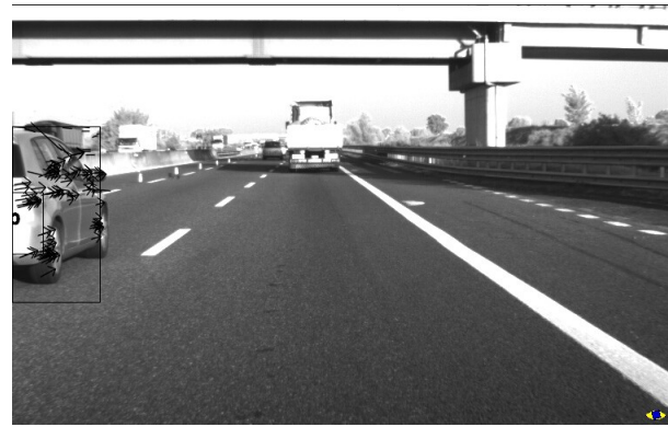
Figure 7. Radar detection of a vehicle outside the field of view of the camera and optical flow positive detection.
