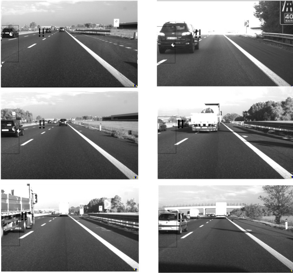
Figure 8. Results for daylight condition. Search window is highlighted in back. A signal is triggered to warn the driver that there is a vehicle overtaking. If the signal is showing a black “!!” symbol.
