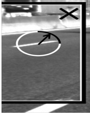
Figure 5. Feature movement angle that fits overtaking vehicle constraints (in black) and not fit (in white).
