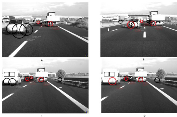
Figure 2. A and C the vehicles has raw data detection (on black) but no detection from the ECU (highlighted in red ). After the vehicles are completely overtaking they are detected (B and D) by the ECU algorithm. There are situations where even after totally overtaking the vehicle is not detected after several frames (A and B).
