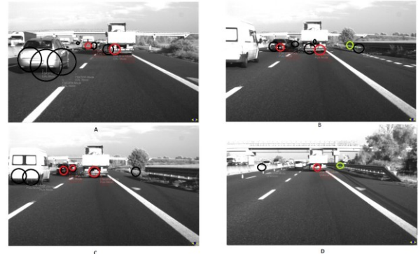
Figure 6. Raw radar data detections on black, vehicles detection given by the ECU on red, and not moving detections on green. A Multiple detections for a single vehicle. B Misdetection of an overtaking car. C and D not vehicles detections at laterals.
