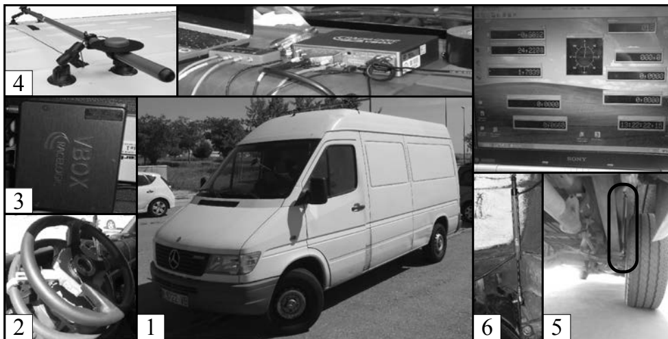
Figure 4. Experimental setup on a test vehicle. (1) Mercedes Sprinter. (2) Steering angle sensor MSW 250 Nm. (3) VBox 3i dual antenna data logger. (4) GPS antennas. (5) LVDT MNT potentiometer. (6) SA-LP075 potentiometer.
