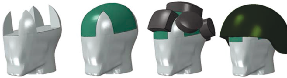
Fig. 8. Ballistic dummy headform with a clay insert. From left to right: the dummy head, headform with clay embedded, including the foams, and the final assembly of the helmet on the dummy headform.
