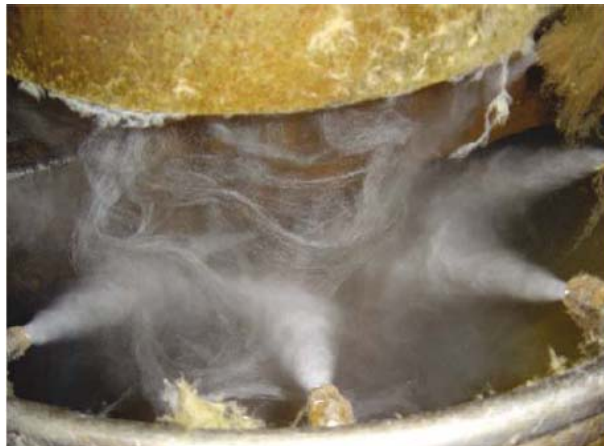
Figure 6.1 – Spraying of binder over fibers just after fiberization [2]
