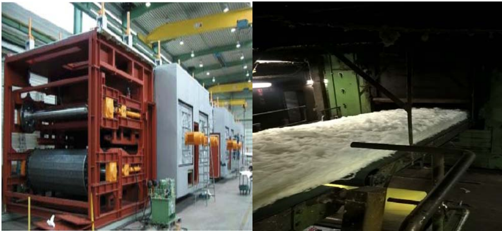
Figure 6.2 – Curing oven for mineral wool manufacturing [2] (left) and mineral wool mat entering in the curing oven (right)
