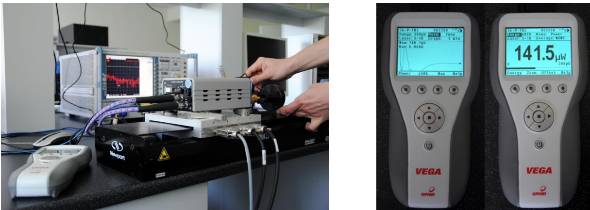
Fig. 11. Direct measurement by Ophir VEGA [10]
