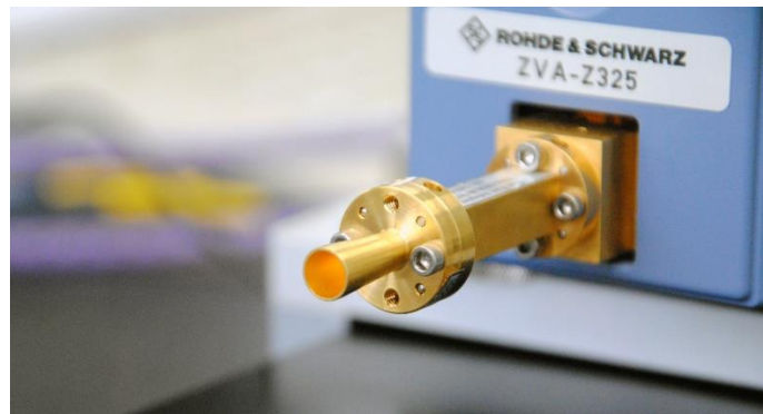
Fig. 9. Circular horn antenna [10]
