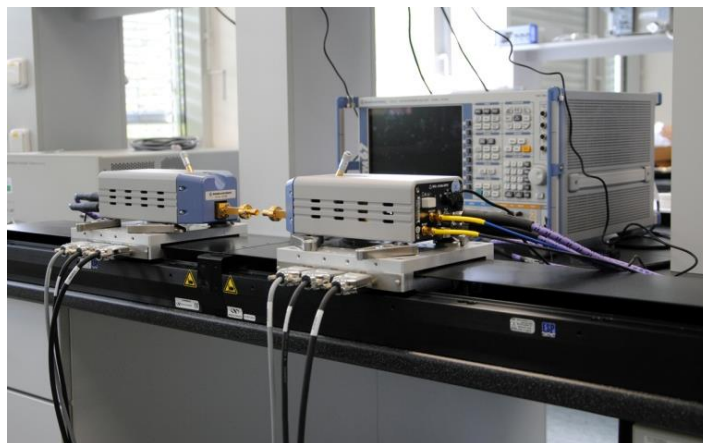
Fig. 1. Vector network analyzer with frequency converters [10]
