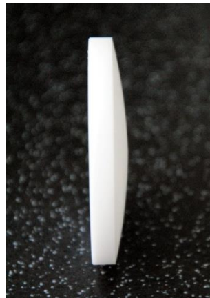
Fig. 5. Manufactured plano-convex Teflon lens [10]
