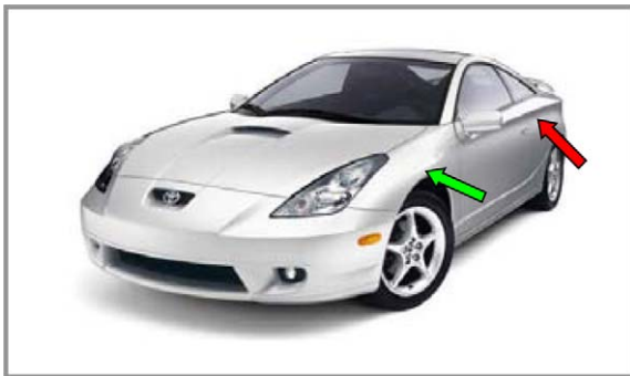
Fig. 2. Example of an accent line with change of continuity along itself (the green arrow points to G^1 continuity, while the red one to G^0 continuity) (courtesy of Toyota).
