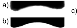
Fig.6. Tool profiles. a) Experimentation b) Simulation c) Profiles differences. black: simulation extra volume.
