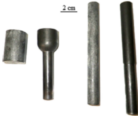
Fig. 2. Photograph showing the billet and the forged specimen, for both batches. Left: 75% reduced cross-section. Right: 18% reduced cross-section. The specimen heads are not yet machined. Photo credit: Gevelot Company.
