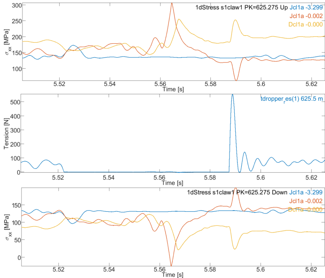
Figure 17: Up (resp. Down): Uniaxial beam stresses at upper (resp. lower) line of CW (blue: far away from junction claw, red: just before junction claw, orange: just after dropper claw). Middle: Tension in dropper. Junction claw @625.275m.
