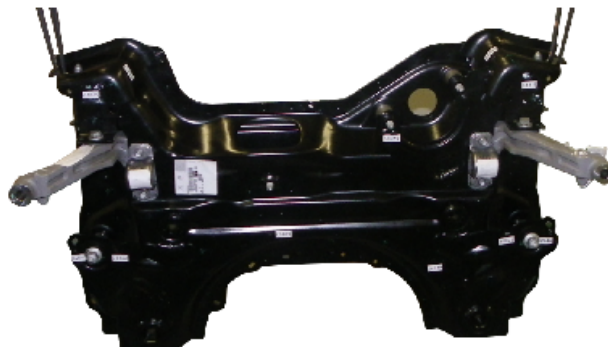
Figure 1: Engine cradle used as test case.
