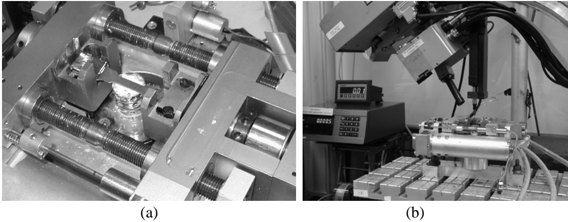
Fig1. In-situ tensile test device. (a) Micro tensile machine and cooler device. (b) X-Ray diffractometer.
