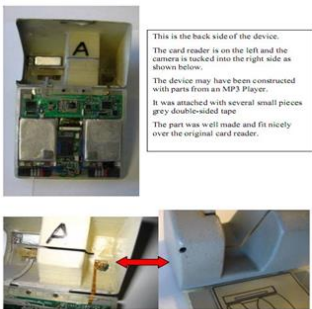
Figure 4: ATM skimming device (false card slot overlay)
