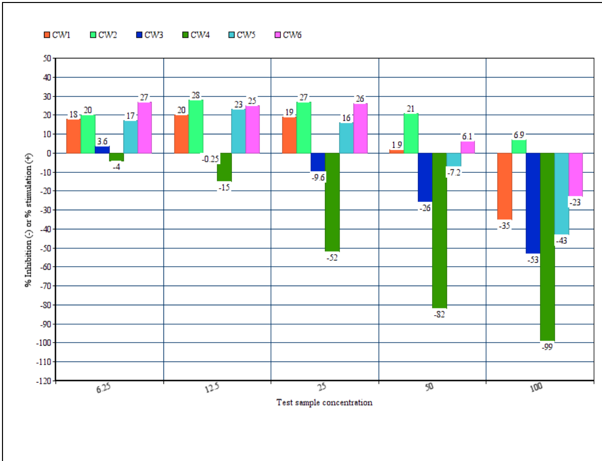
Figure 26: Thirty minutes Vibrio fischeri bioluminescent toxicity test results
