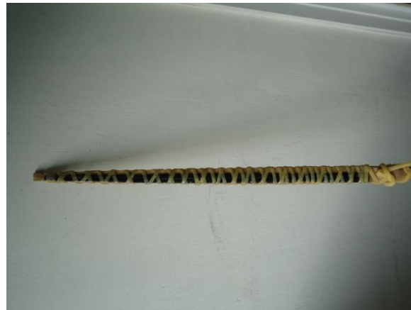
Figure 6.18 Gluing horn lath to belly of bow limb, two thirds complete. Note surgical tubing used as clamping.
