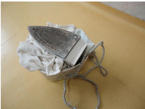
Figure 6.9 Inverted iron, placed in a corning ware pot and stabilized with dish towels.
