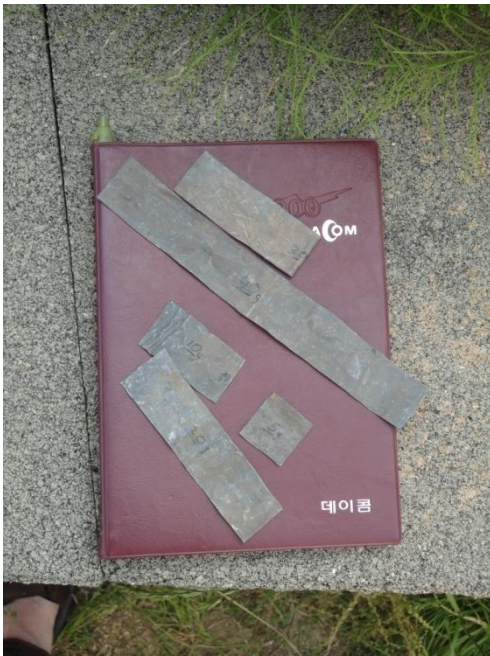
Figure 6.42 Lead Strips 5g, 10g, 20g, 30g and 40g in mass.
