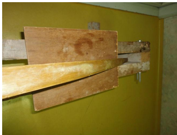
Figure 6.12 Finished, partially dried sinew backing.
