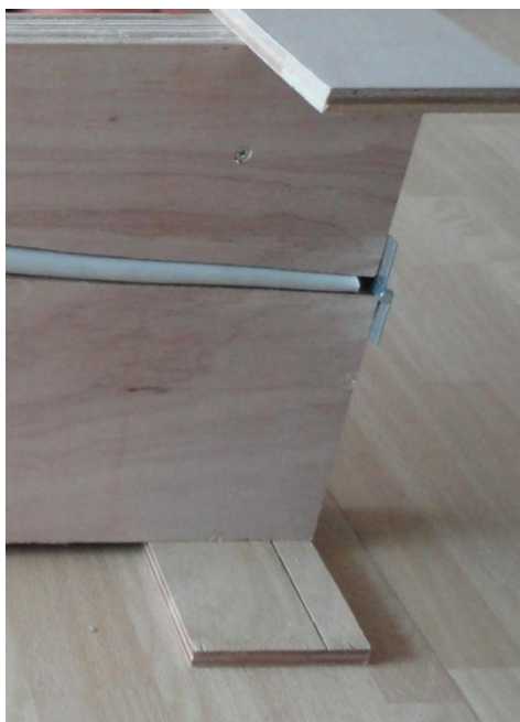
Figure 5.5 Close-up of jig hinge.
