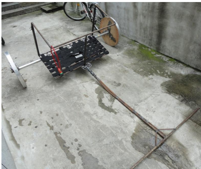
Figure 5.15 Assembled chariot. Note floor panel made of woven nylon webbing.
