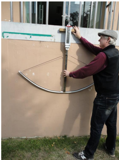
Figure 6.1 Author measuring the draw weight of a heat-molded PVC bow.
