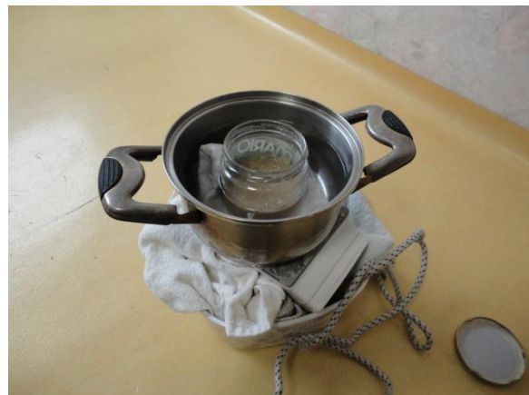
Figure 6.10 Complete double boiler assembly. Note the cloth under the jar of glue preventing it from coming in direct contact with the bottom of the pot.
