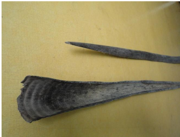
Figure 6.17 Gemsbok horn halves split lengthwise. Note radial arc.
