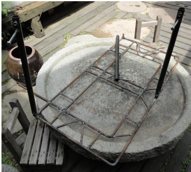
Figure 5.13 Chariot box base. Note the removable upright sleeves (two attached) allowing for an adjustable railing height.
