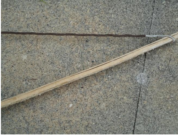
Figure 6.13 Close-up side view of composite bow. Note the glue line between the main body of the bow and the added wood slat on the belly.
