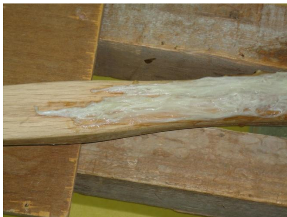
Figure 6.11 Close-up of partially laid sinew backing.
