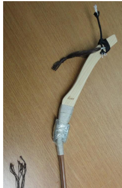
Figure 6.43 Bow with broken string and added mass. Note the folded strip of lead taped to both front and back.
