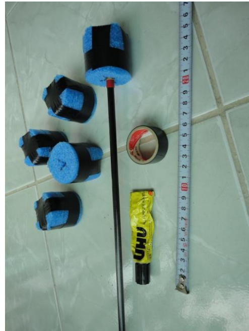
Figure 5.10 Assembled safety tips and completed arrow.
