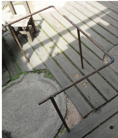
Figure 5.14 Chariot box railing. The three vertical members slide into the sleeves shown in figure 5.14.
