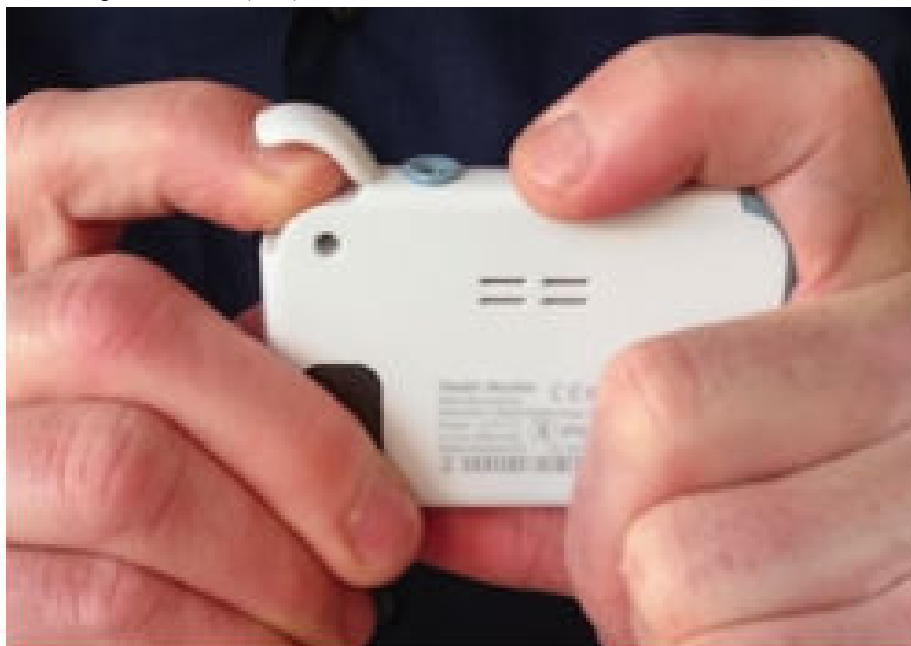
Figure 3. Checkme position during measurement (back).
