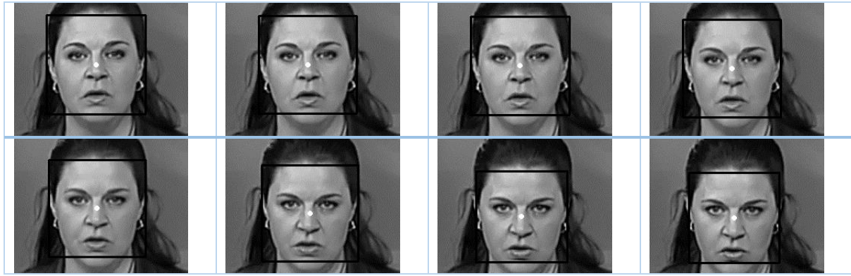
Figure 1. Faces detected in successive frames during a head movement. The black square is the detected face, the white dot (at the center of the square) is the x-y coordinate we use.
