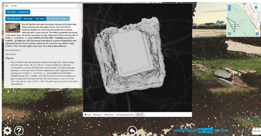
Figure 6. Snapshot of the web viewer showing a point cloud of a selected site on top of the background point cloud, a mesh on a different 3D scene and the site information box with attributive data of the selected site.
