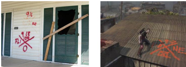
Figure 24 – FEMA marking system 64
