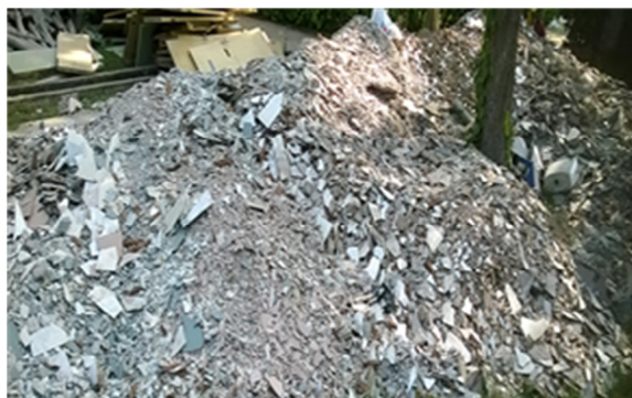
Fig. 1a Ceramic wall tiles wastes from a demolition site at Ota, Nigeria.
