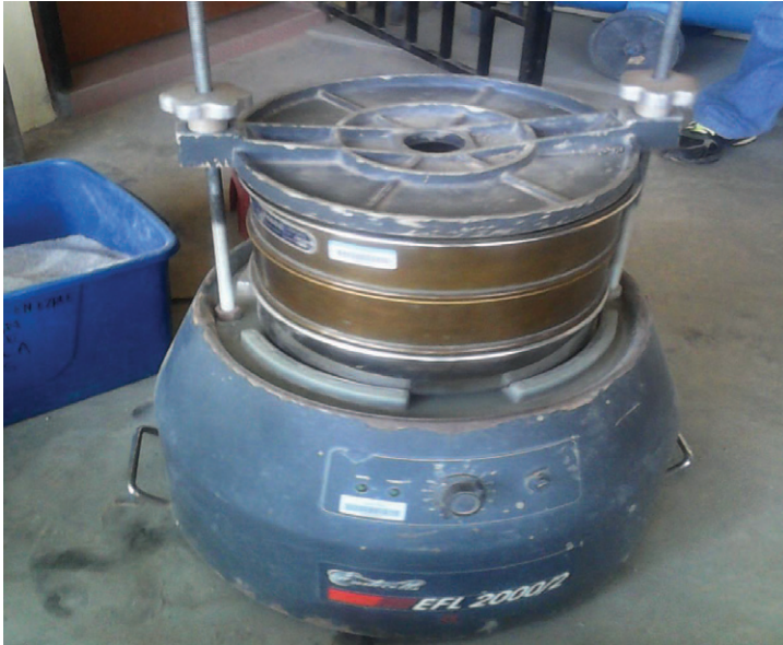
Figure 3.8 Sieve shaker machine sieving crushed rock samples through sieve mesh of 250 µm.
