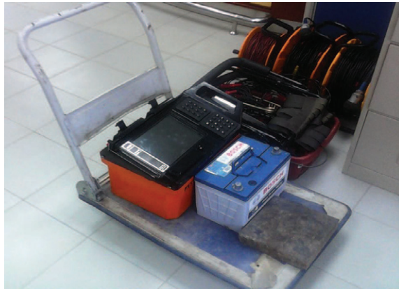
Figure 3.3 Campus OmegaC2 Terrameter
