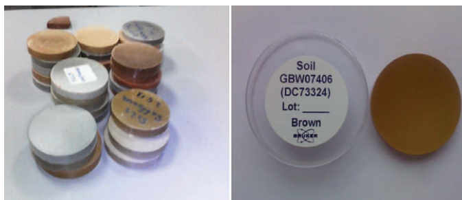
Figure 3.18 Prepared rock samples for X-ray analysis and the standard reference material
