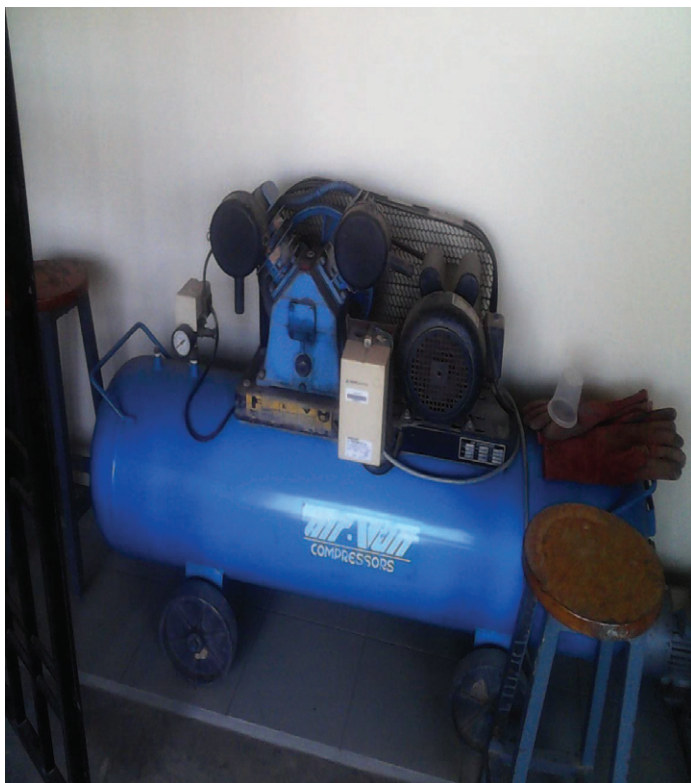
Figure 3.9 The high pressure air flushing machine that keeps the sieve mesh and crushing machine clean at each use to avoid cross-contamination of rock samples.
