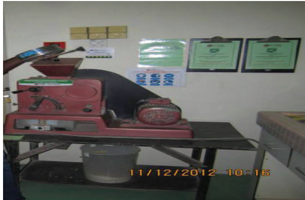
Figure 3.7 The rock sample crushing machine was set at 250 \mu m sizes in Applied Geophysics Lab., UTM (made by Bico Pulverizer MFD, Bico Inc. UA Burbank California)
