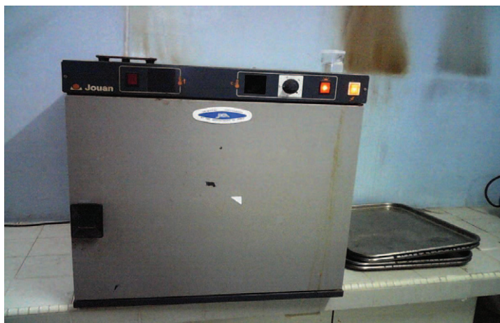
Figure 3.6 Oven for drying the rock samples at Nuclear Lab. UTM (made of Jouan by Japan)
