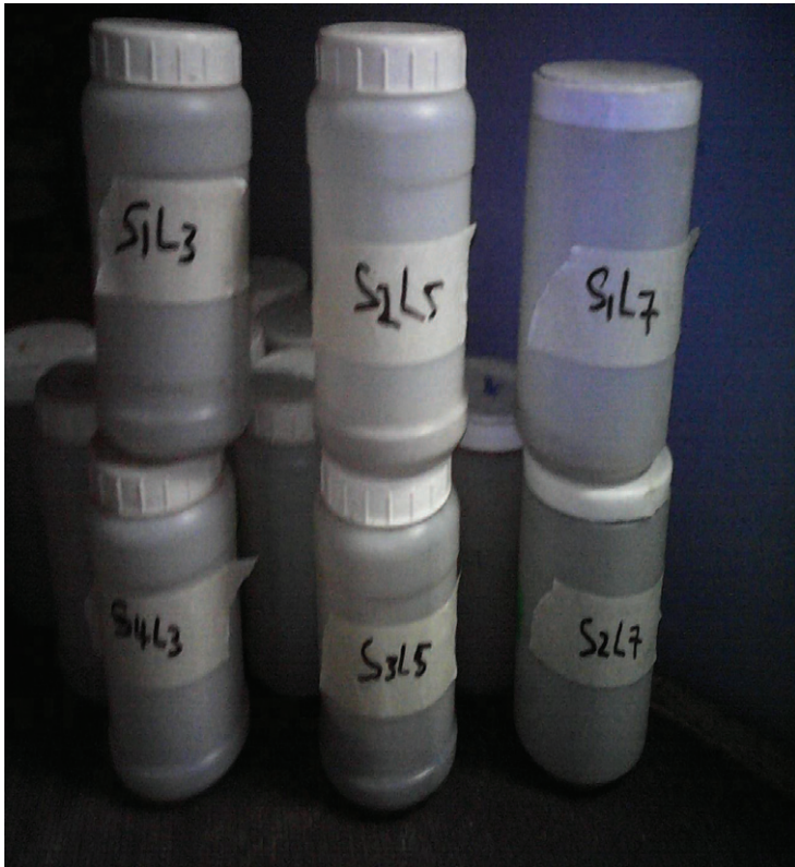
Figure 3.10 Temporary plastic bottle containing each sieved rock sample labeled according to sample site and layers.
