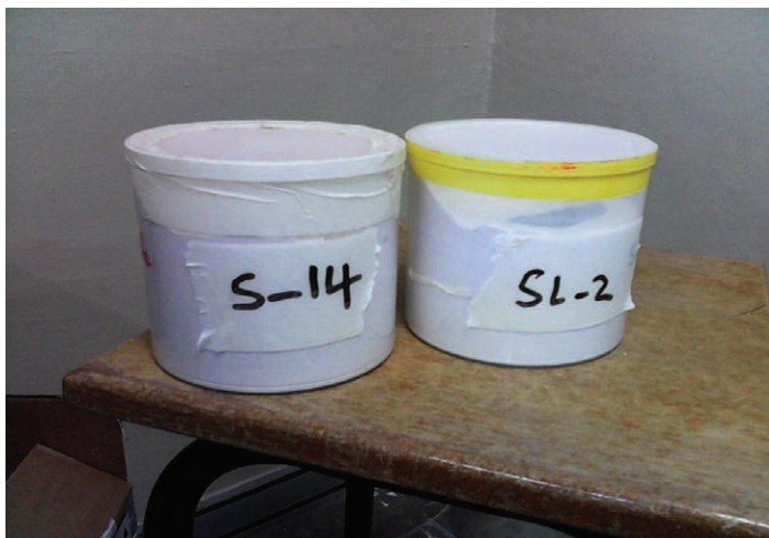
Figure 3.14 Standard Sample (IAEA) for S-14 (Thorium ore) and SL-2 (Lake sediment) prepared for gamma analysis
