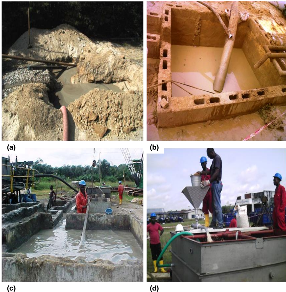
Figure 3. Types of mud pit used during the drilling process (a) unlined pit (b) lined pit (c) elevated Pits (d) mud tanks.
