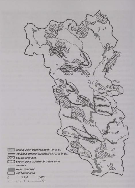
Figure 7 Delimiting of areas found to be in poor ecohydrological condition in the Košínský Brook basin
