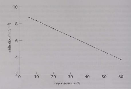
Figure 2: The trend of infiltration over the South Makár study area
