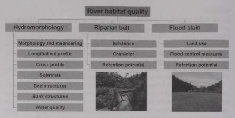
Figure 1: Scheme of the river habitat quality assessment according to EcoRivHab method
