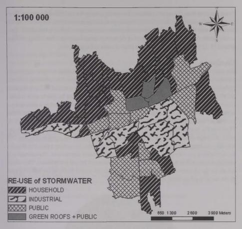
Figure 3: The most adequate techniques for the re-use of rainwater over the city of Pécs
