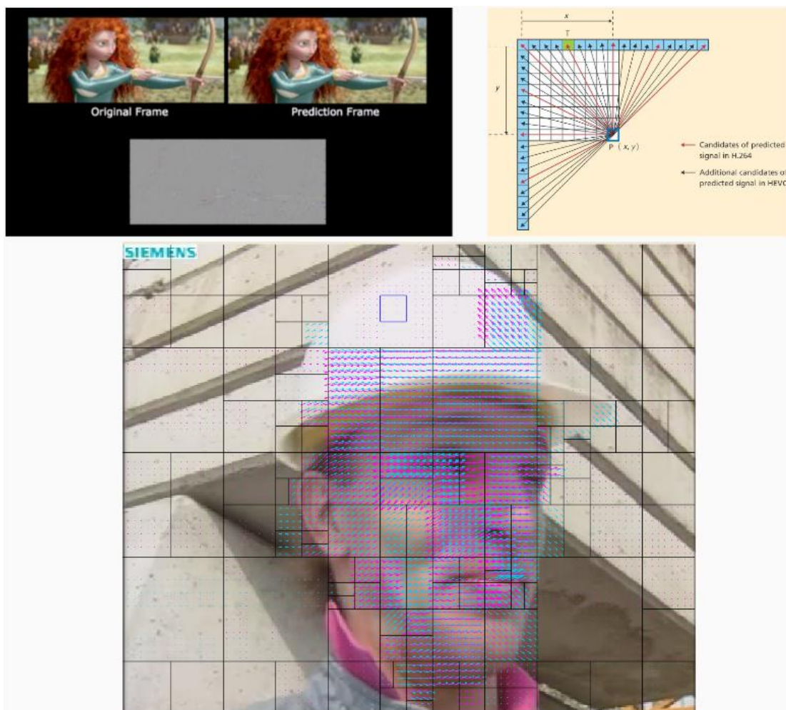
Figure 2.10: HEVC encoder prediction, source : [6]
