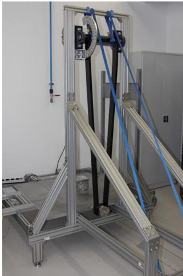
Figure 2.2: Shock testing system at Tartu Observatory's space technology laboratory
