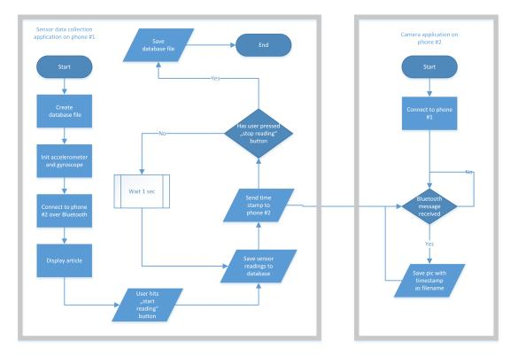
Figure 5.3: Data collection system program flow chart
