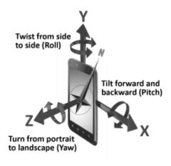
Figure 2.5: Phone gyroscope [4]
