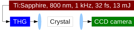
Figure 3.1: Experimental setup at CEA-Saclay. The first and second lenses have the focal lengths of 100 cm and 5 cm, respectively. Spot size on the crystal is 102 \mu\text{m} .
