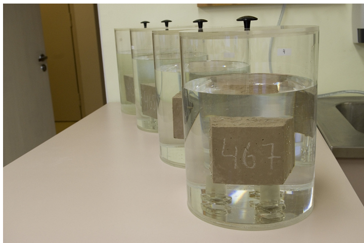
Figure 5. Tank leaching test for oil shale ash-based monoliths at National Institute of Chemical Physics and Biophysics in 2013.
