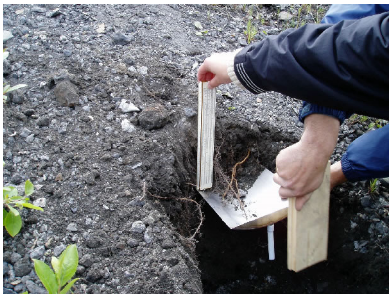
Figure 3. Installation of a sampler at the closed site of the spent shale deposit.
