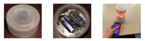
**Figure 7.3: Light cylinders.** The cylinders were built of semi-transparent acrylic and equipped with an Arduino board and LEDs. Colors of individual cylinders are changed via a smartphone app.
