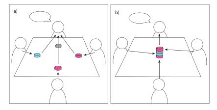
**Figure 7.2: Study setup.** a) Light cylinders are placed in front of each group member to provide identifiable feedback to the current speaker. b) Light cylinders are stacked on top of each other in the middle of the table and feedback is sent to a randomly selected cylinder to provide anonymous feedback.
