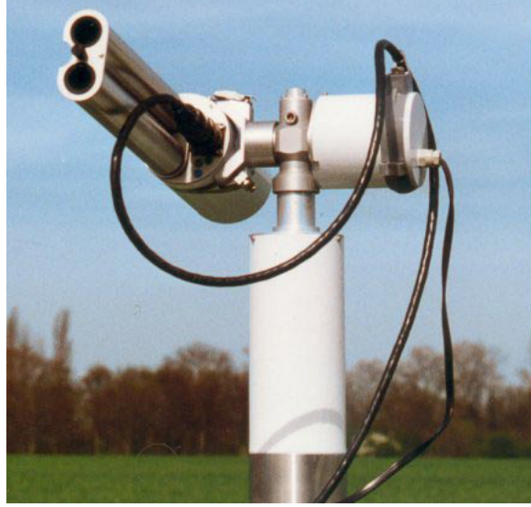
Figure 3.3: Sonnenphotometer CE 318 des Herstellers Cimel Electronique (CIMEL Electronique, 2000-10-09)
