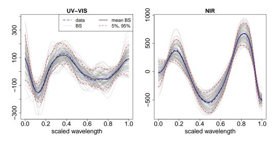
Figure 3.6: Estimated coefficient functions for the model on fossil fuels. Coefficient estimates for the effects  $\hat{\beta}_j(s_j), j \in \{1, 2\}$ , of the two spectra. The gray lines show the estimates in the 50 bootstrap folds, the black line gives the mean estimated coefficient over the bootstrap folds, the dashed red lines point-wise 5% and 95% values; the long-dashed blue lines give the estimated coefficients for the model on the whole dataset.
