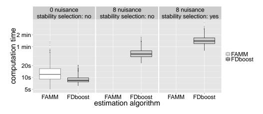
Figure C.6: Computation time for FAMM and boosting in simulated data. The computation time for FAMM and boosting with zero or eight extra nuisance variables. In the presence of nuisance variables boosting is used with and without stability selection. Note that the computations for boosting were performed on ten cores, whereas for FAMM only one core was used.
