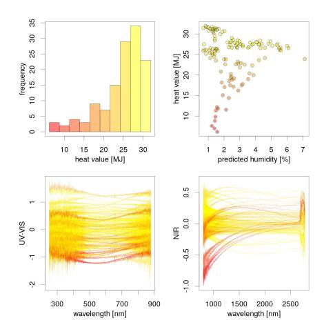
Figure 3.4: Spectral data of fossil fuels. The coloring of all plots is according to the heat value in MJ, with red meaning low heat value and yellow meaning high heat value. The histogram at the top left can be used as a legend. The scatter plot at the top right shows the heat value depending on the predicted humidity. The lower panel shows the UV-VIS and the NIR spectra colored according to the heat value.
