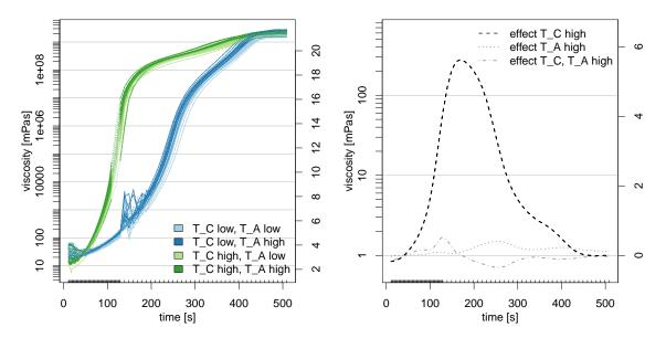
Figure 3.3: Viscosity over time and estimated coefficient functions. On the left hand side the viscosity measures are plotted over time with temperature of tools  $(T_C)$  and temperature of resin  $(T_A)$  color-coded. On the right hand side the coefficient functions are plotted.
