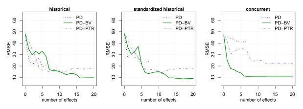
Figure 4.4: Predictive power of functional models for the fermentation data. Prediction error (RMSE) for each model type–historical, standardized and concurrent model (from left to right)–and covariate set (PD, PD-BV and PD-PTR) as a function of the number of variables in the model computed over CCV.
