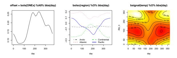
Figure 6.3: Coefficient estimates of the Canadian weather data model with optimal number of boosting iterations. The smooth intercept (left), the region-specific effects (middle) and the effect of temperature (right) are given. The regions are color-coded. The variable t is denoted by 'day'; the variable s is denoted by 'day\_s'.
