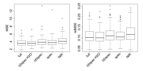
Figure 3.5: Predictive power of models for the heat value of fossil fuels. MSE and relMSE for models with different effects: the model with all effects (*full*), with all the main effects (*(d)spec H2O*), the effects of both spectra and their derivatives (*(d)spec*), the effects of both spectra (*spec*) and the effects of the NIR spectrum (*NIR*).
