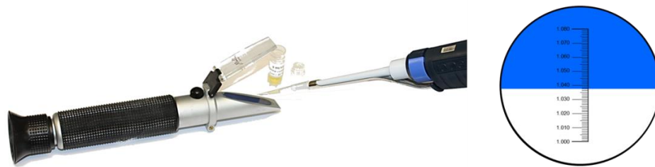
Fig. S245. Refractometric determination of the urine density.
