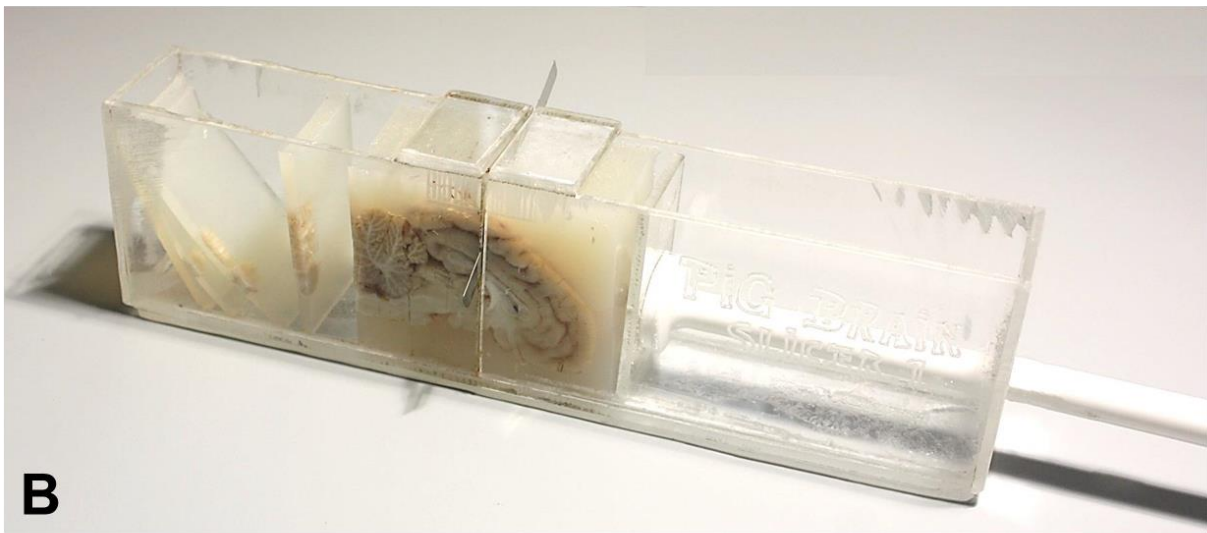
Fig. S137. Serial sectioning of agar-embedded brain tissue in a self-constructed tissue slicer. A schematic illustration ( A ) and image ( B ) of brain sections.
